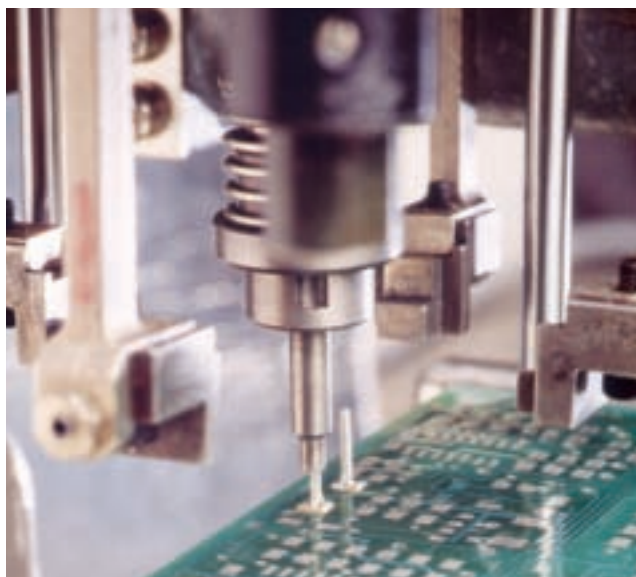
Odd - shaped parts can be assembled in-line on existing placement equipment.
