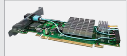
PCle®-over-Fiber adaptor card (PCOA) supports transparent and non-transparent bridge links using PCUO FireFly™
