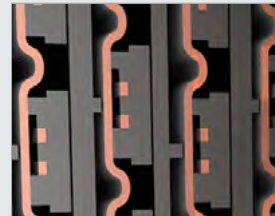
Staggered, differential pairs
