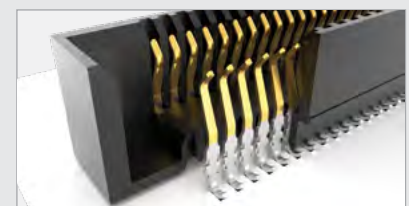
Signal integrity optimized Edge Rate® contact system reduces broadside coupling
