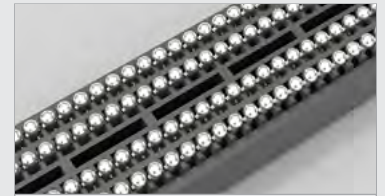
Solder ball technology for simplified processing and self aligning
