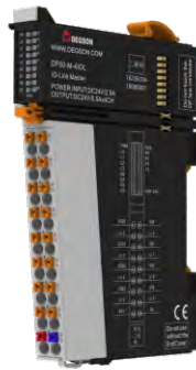
IO-Link communication module, 4 channels
