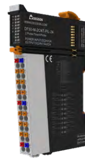
5V Pulse counting module,2 channel
