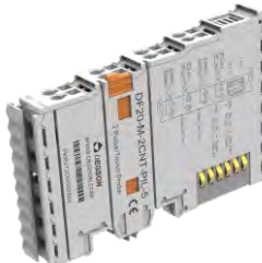
Pulse counting module, 2 port,5V
