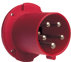
For panel mounting with straight flange, Type ...BU... 63 A, IP44
