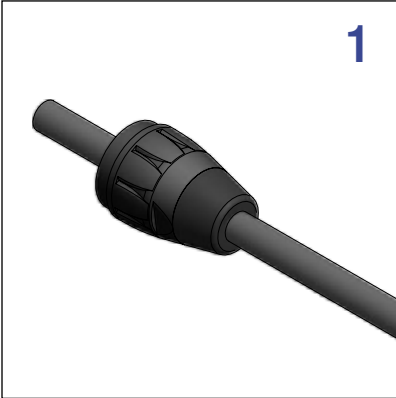
Slide the nut onto the cable
