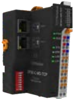
ModbusTCP, 2 RJ45, extensible 32 modules, 24VDC
