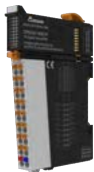
Digital output module, 16 ports, PNP, 24VDC
